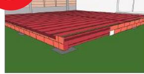
Attach brick skirt and modular brick walls to steel base and finish by fixing the bridging tiles in place.
