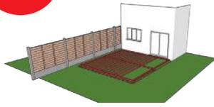
Lay down the steel base and level using the adjustable legs then fix to the house wall.
